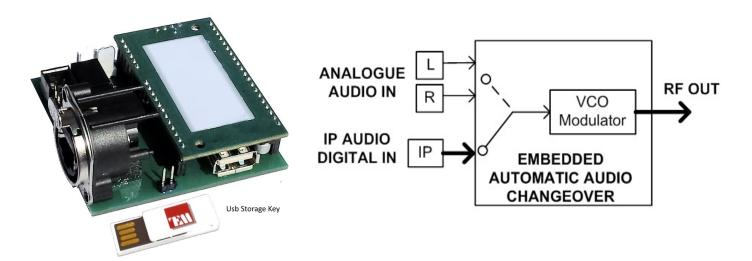
New IP Audio Decoder board, code nr. 13M31940, is a very helpful solution to decode your audio program from IP network.
