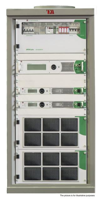
OPERA plus 10KW FM 87,5÷108MHz transmitter uses 2x5000W amplifier with 6^ generation LDMOS technology, 65:1 VSWR and 6x3500W Hot Pluggable Power Supplies.
