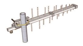
Suitable for particularly unfavorable environmental conditions. The antenna is made of tubular aluminum . 2mm thick pre-galvanized steel fixing bracket to the pole, positioned in the rear part of the antenna. The antenna can be mounted in horizontal and vertical polarization. The antenna are supplied fully assembled.
